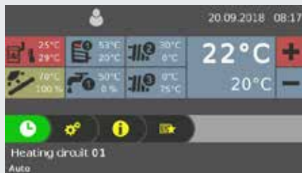
Fig. 1 General overview of heating circuit (start screen)
